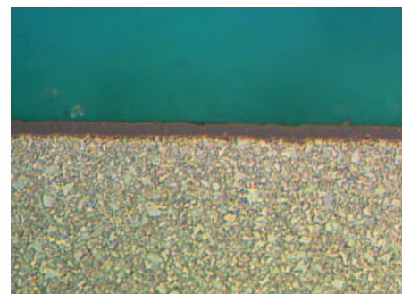
Cross-section view of PVD coating
