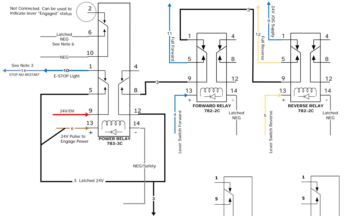
Note 1: Black Line is 24V supply available when 24V power is latched. This is SOURCE LOGIC. Relays and logic terminals are energized using the External 24V Power Supply. The VFD 24V power is NOT used.
