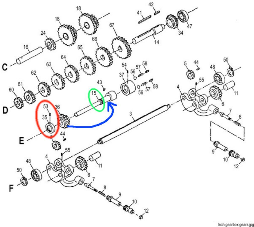
The shaft in question is “E” in the drawing. Although the drawing shows a collar with set screw (circled in red) holding the shaft in position, that element does not exist. The gear #36 sits further up the shaft as shown with the blue arrow, and a snap ring (circled in green) holds
