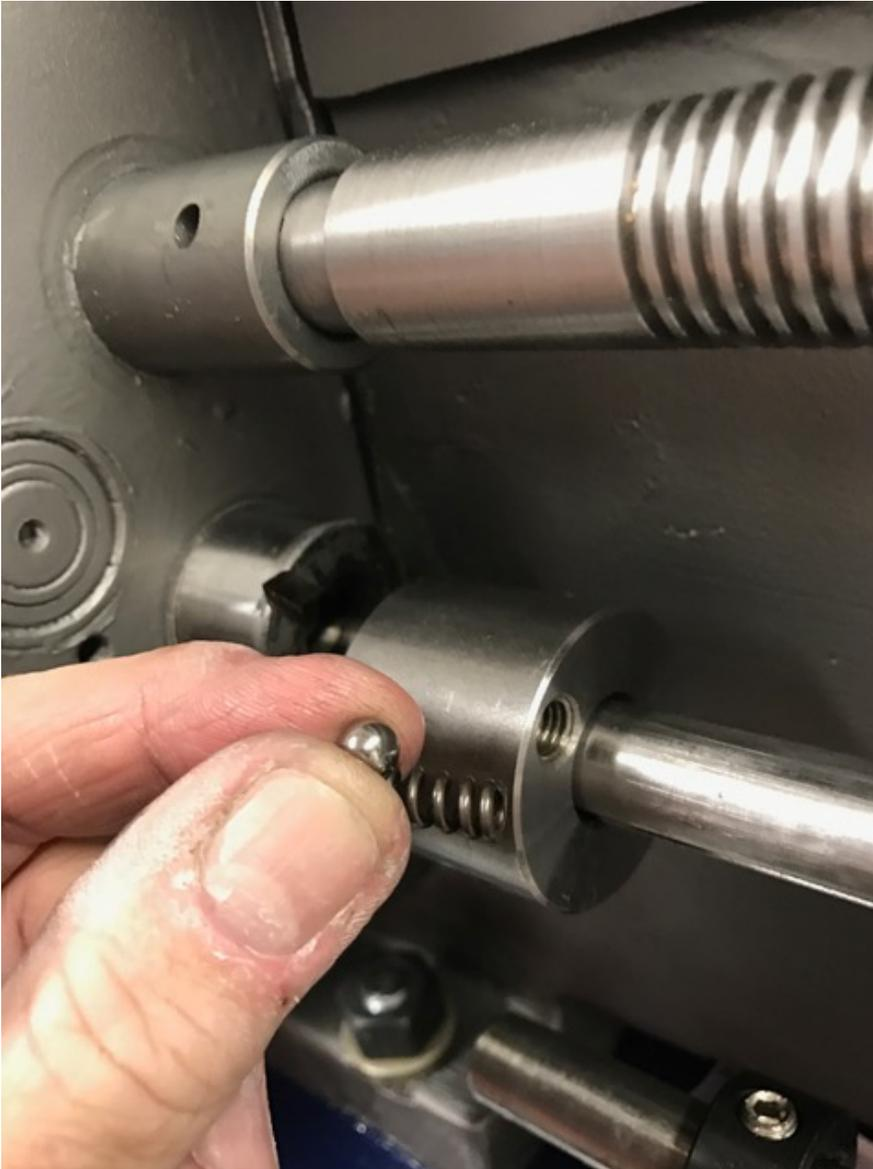
The clutch comprises a pair of spring loaded steel balls bearing on a detent disc driven by the Norton gear-box. Spring pressure is adjusted by two set screws on either side of the feed shaft, arrowed. Setting the spring pressure is a process of aiming for the best compromise between too high and too low, which might mean unexpected stopping for no good reason.
