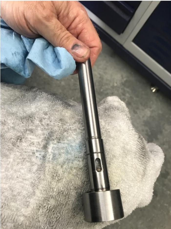
The shaft is supported with a bronze bushing with oil galleries around the inside of the bushing. That bushing, and the part of the shaft that was in the bushing was gunked up with something that looked like tar. This was the source of the friction that was keeping the shaft from spinning freely, and which got worse as the bearing surfaces got hot. I suspect that tar-
