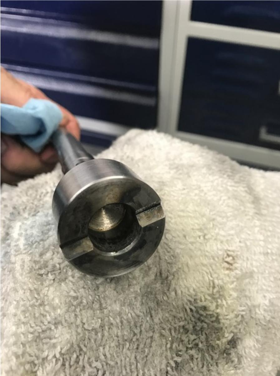
The outside end of that shaft (with the two V-shaped notches) is the clutch (ball bearings on springs) that will give way if the feed shaft is stalled downstream.
