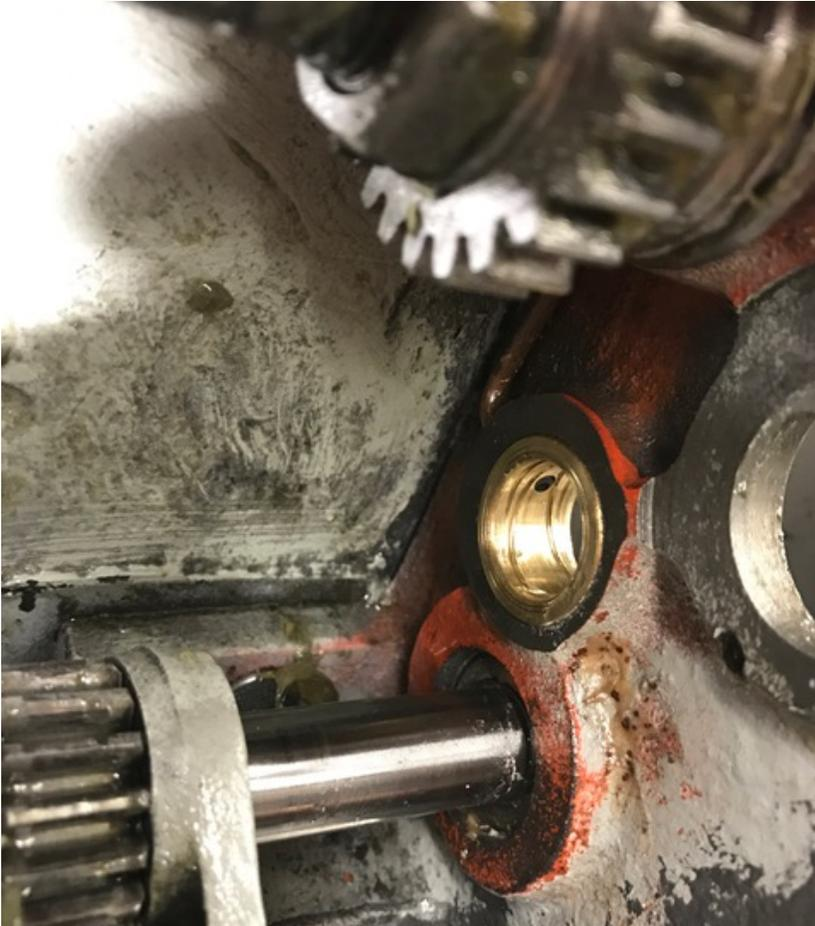
By the way, that bronze bushing is lubed by oil coming down from the galleries above via a small copper tube to the back where you see the hole in the bushing.
