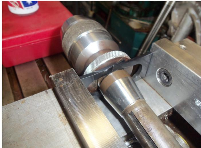
The biggest issue in using a Morse taper on a mill is that removing the tool from the spindle requires driving a drift into the back end and side of the spindle forcing the tool outward. A better way was required to secure the tapered tool end into the tapered spindle socket and to facilitate removal.
