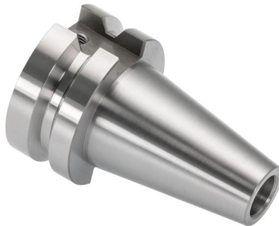
The taper is shorter, and the angle is more severe when compared to the R8, which makes this taper self-releasing when released from the spindle. The torque drive mechanism is via the two slots on the side of the tool holder – the spindle has two dogs that protrude outward to mesh with those slots and push the torque into the tool holder. The small end of this taper is a threaded hole, much like the R8.
