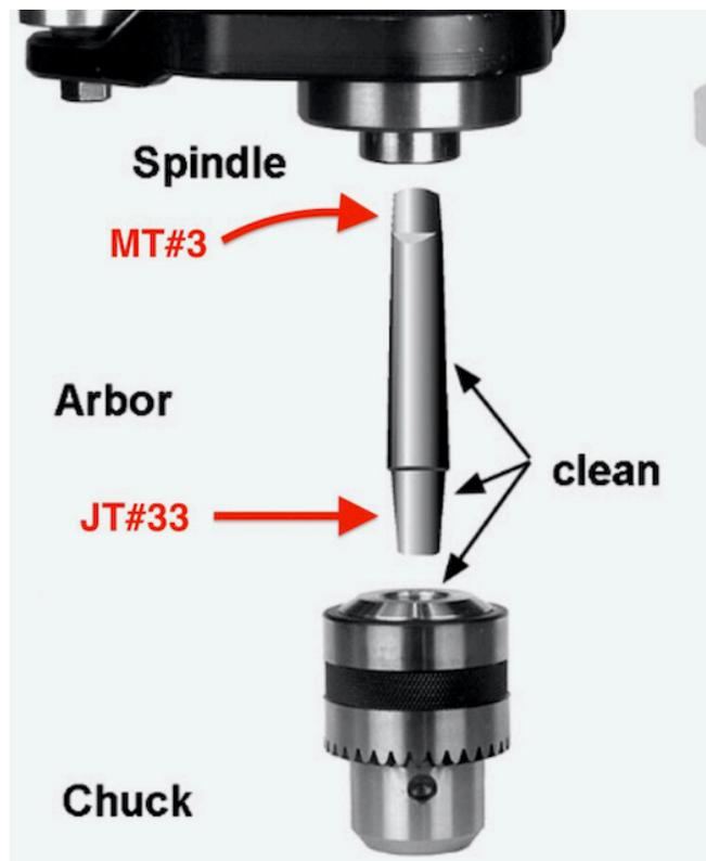
A tool or arbor with a Morse taper, may also have a flat section at the narrow end of the taper called a tang. When the tool or arbor is seated in the spindle of a machine, the taper secures the tool from falling out, while the tang will slot into a recess in the spindle to prevent the tool from slipping or twisting loose inside the spindle under extreme torque loads.
