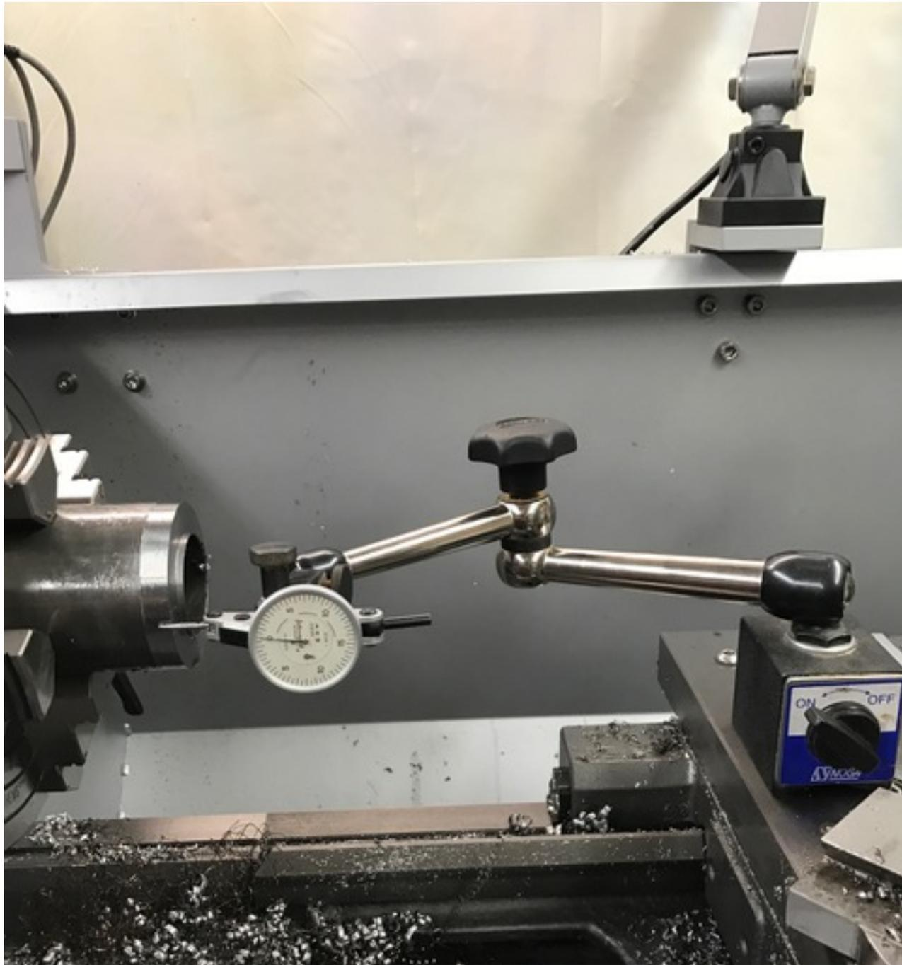
I set the DRO display for the Z axis in Diameter mode and zero out the indicator (just calibrated last month), the DRO and the handwheel dial:
