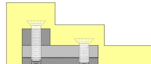
Drill & Tap Chuck for 10-24 screws, 10mm deep twelve (12) locations as shown.
