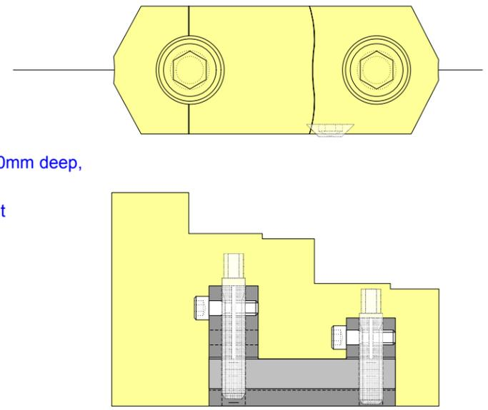
Tap Locations for Clamping Block Screws
