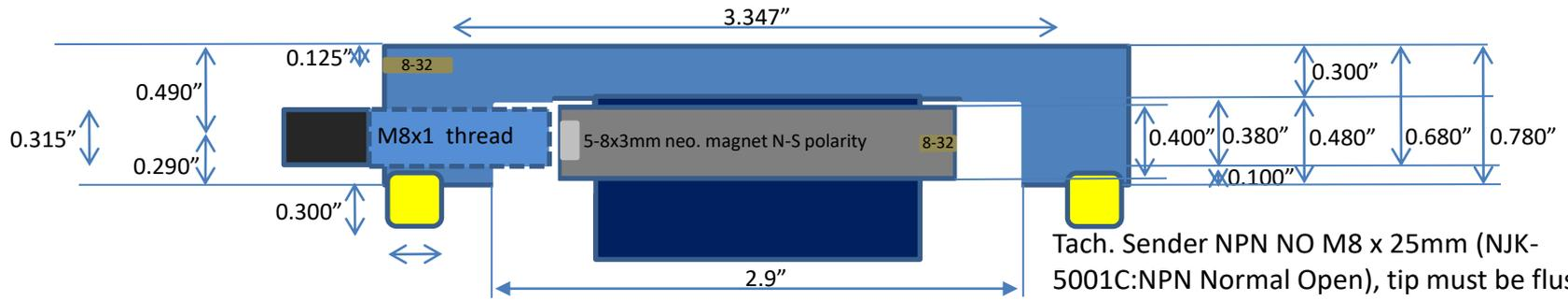
Tach. Sender NPN NO M8 x 25mm (NJK-5001C:NPN Normal Open), tip must be flush with inner 2.3" circle. Check magnet polarity with sender connected to the tach. before installing. LED 100mm ring /cover is a press fit , but can use silicone sealant to seal. Clip off plastic mounting fingers, file small half circle for wires to exit cover.
