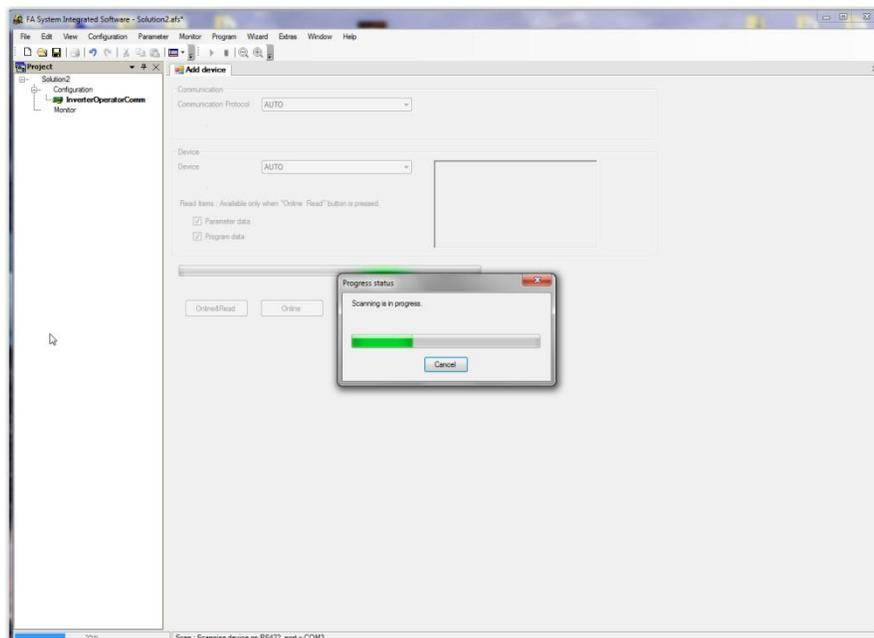
Verifies that it is connected to the WJ200 VFD, click n OK to continue and upload parameters to your PC.
