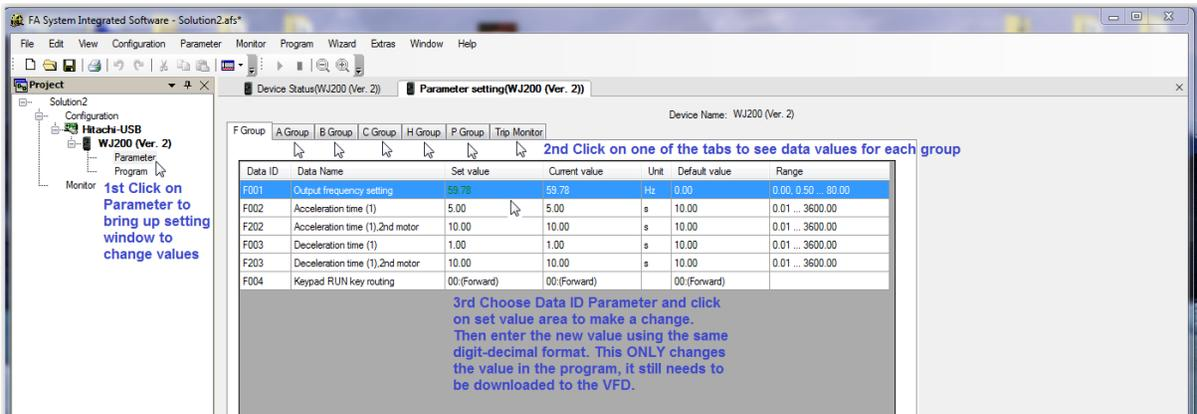
You make changes in the 'Set value' Column, the line(s) will be highlighted to indicate a change(s). The change(s) must then be sent to the VFD.
