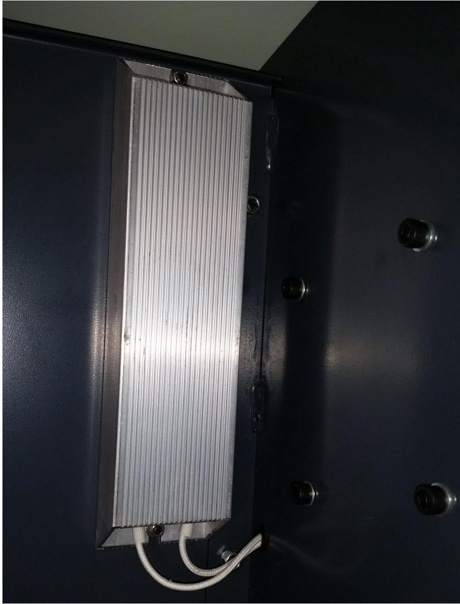
50ohm 500W Braking Resistor (2HP motor). Mount to metal surface. (eBay 50-75ohm, 250-500W)
