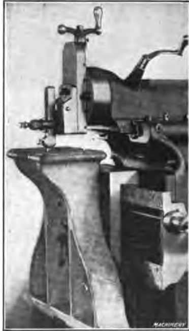
Fig. 5. Table Removed and Casting Clamped to Cross-slide
