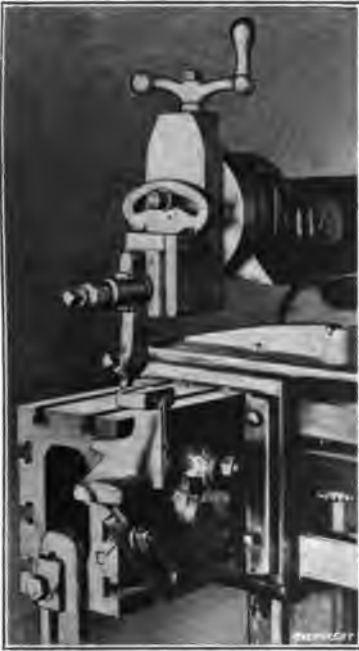
Fig. 4. Casting of Irregular Shape Bolted to Side of Table
