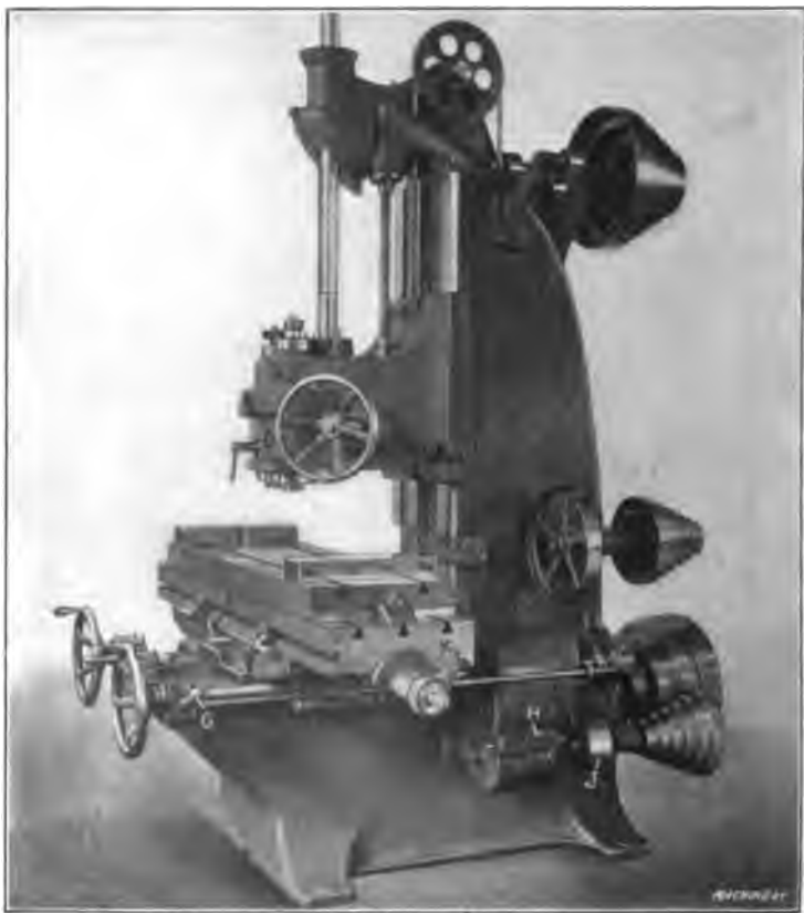
Fig. 12. Pratt & Whitney Two-spindle Die-sinking Machine
