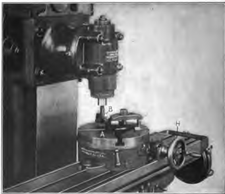
Fig. 21. Combined use of Vertical and Circular Milling Attachments
