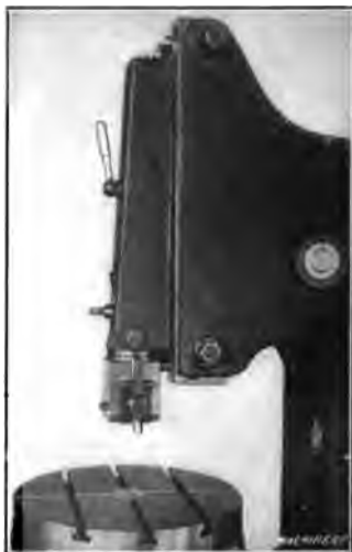
Fig. 13. Ram Head Swiveled through 90 Degrees
