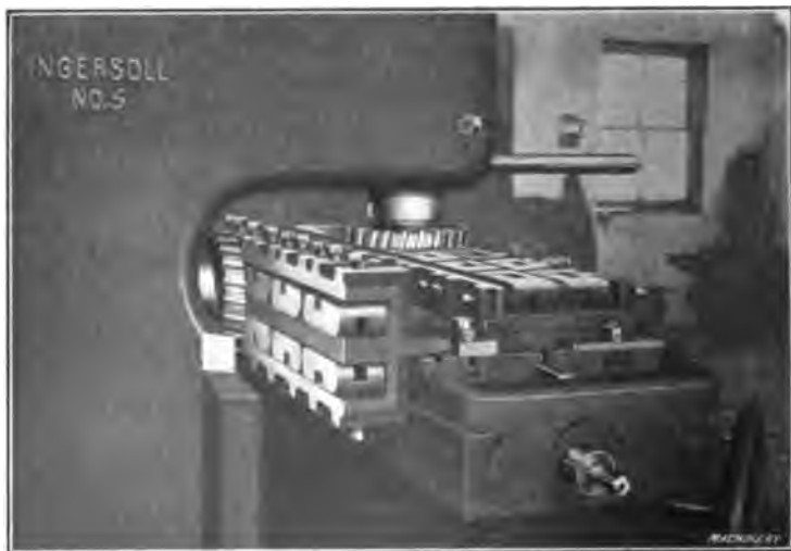
Fig. 14. Ingersoll Combined Horizontal and Vertical Milling Machine — Both Spindles in Operation
