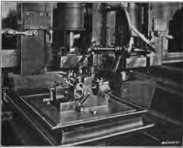
Fig. 20. Profiling Cartridge Guide Slot in Rifle Receiver
