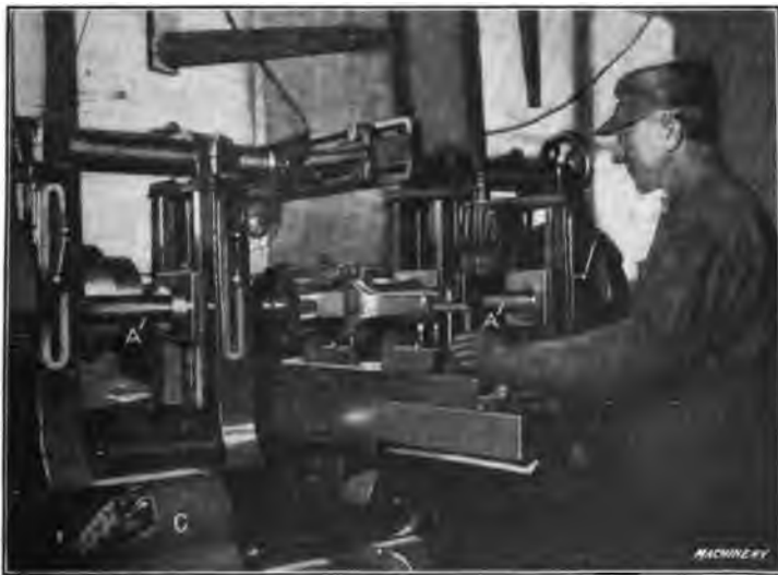
Fig. 40. Example of Parallel Face Milling on a Duplex Machine
