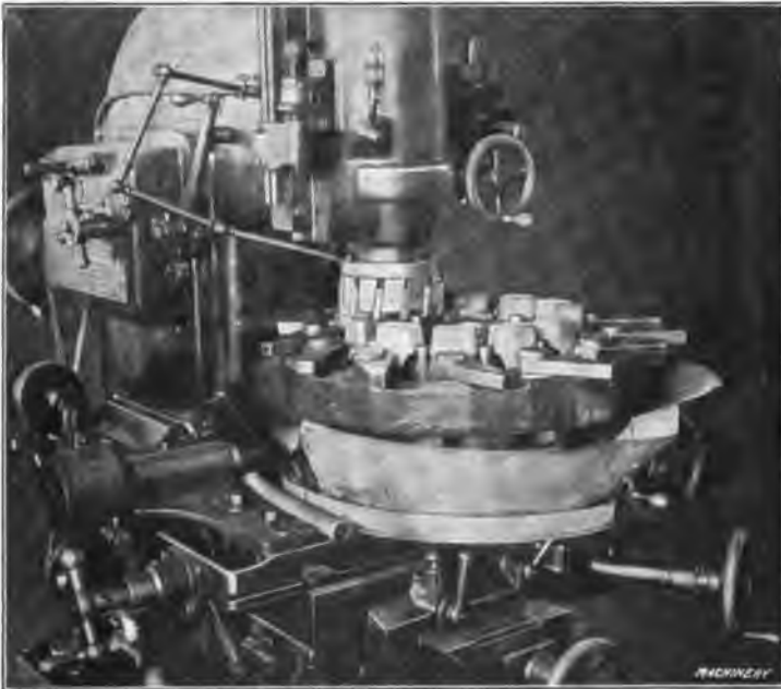
Fig. 10. Continuous Circular Milling Operation
