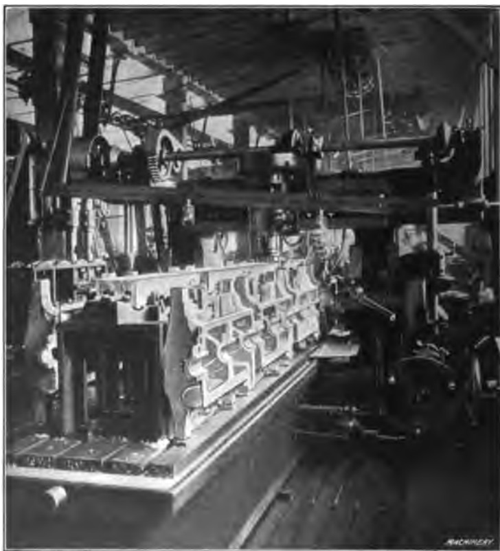
Fig. 37. Three-head Machine Milling Aluminum Castings
