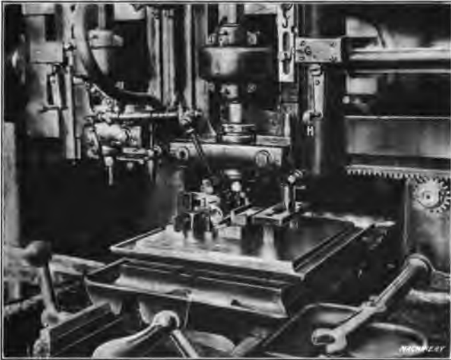
Fig. 21. Profiling Slot in Receiver for Cartridge Ejector
