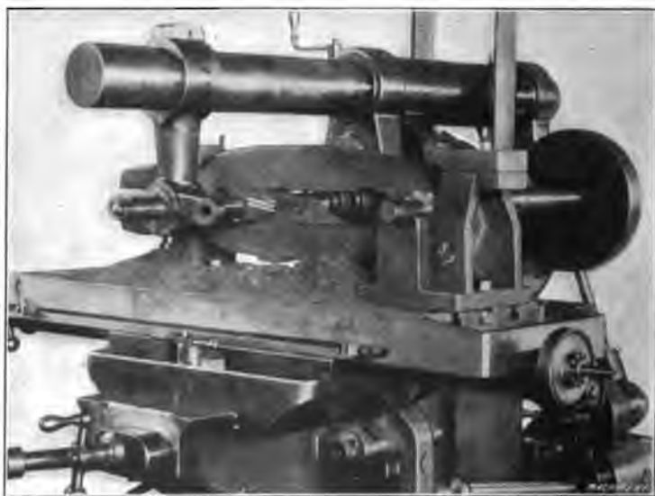
Fig. 18. Milling Slot of Crank-shaper Rocker-arm
