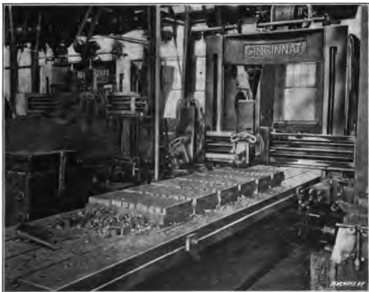
Fig. 52. Planing Teeth in Steel Racks for Frog and Switch Planers
