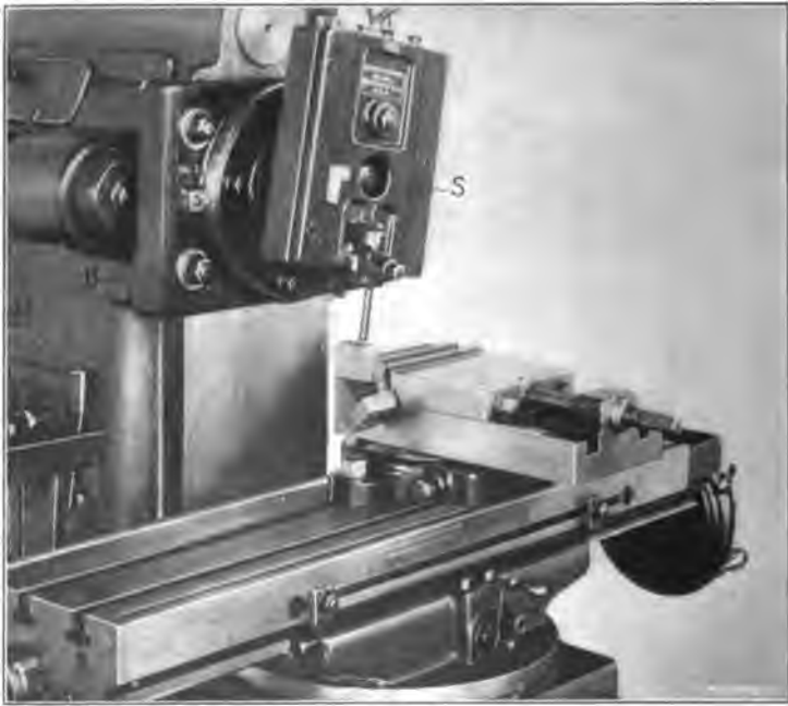
Fig. 19. Slotting Attachment Applied to a Milling Machine
