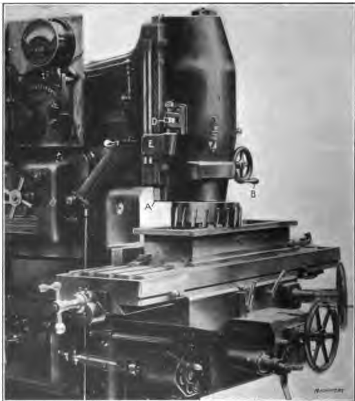
Fig. 7. Finishing Top Surface of a Casting on a Cincinnati Vertical Machine
