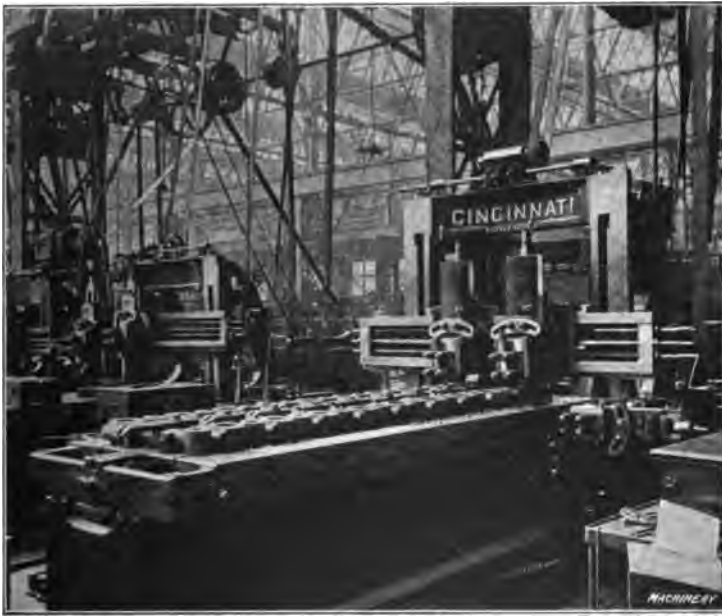
Fig. 42. Twenty Connecting-rods being Planed Simultaneously
