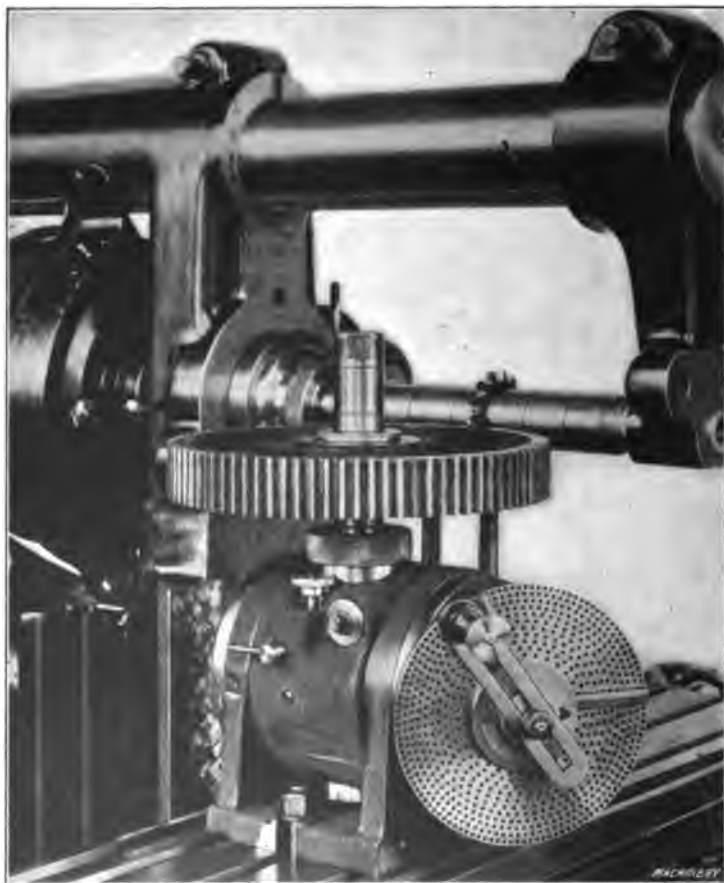
Fig. 6. Dividing Head set in Vertical Position for Cutting Spur Gear 18 inches in Diameter
