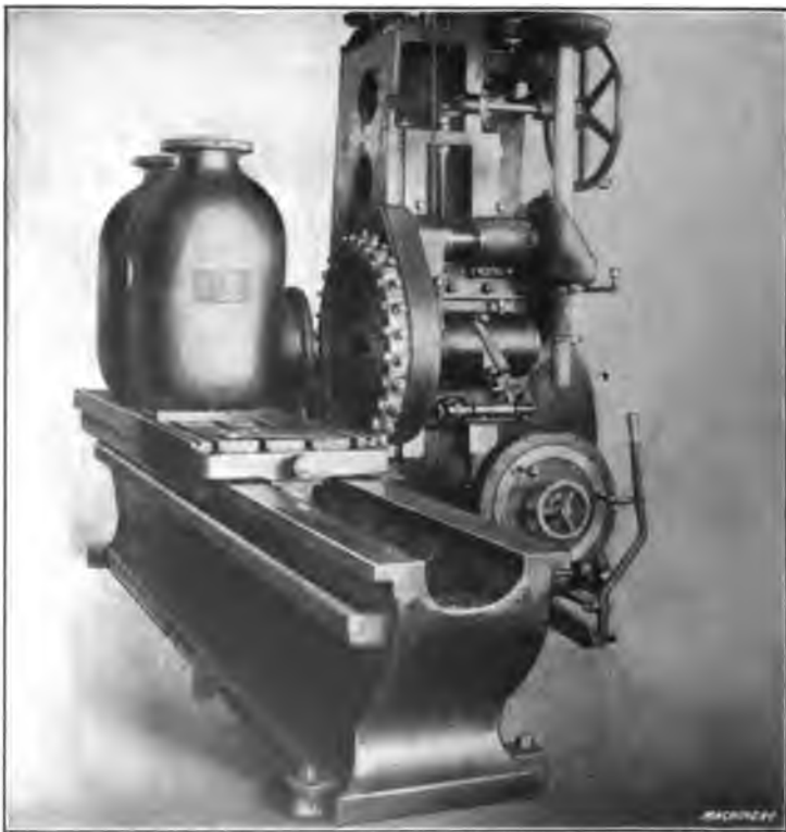
Fig. 39. Open-side Horizontal Milling Machine Facing Pump Castings
