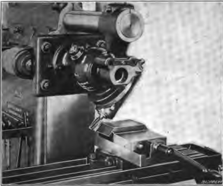
Fig. 18. Vertical Attachment Applied to a Horizontal Milling Machine
