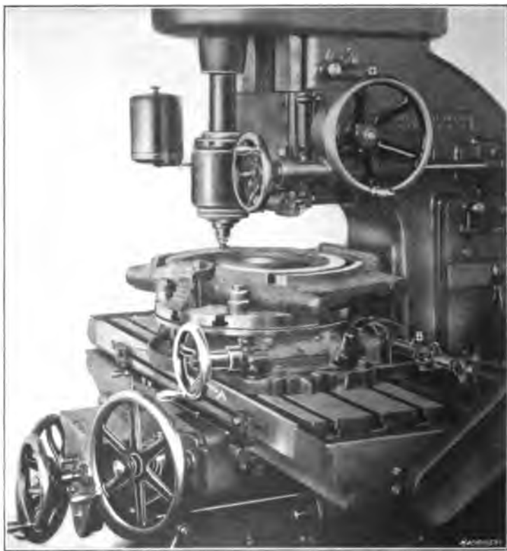
Fig. 3. Milling a Circular T-slot on a Vertical Machine
