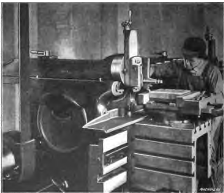
Fig. 3. A Simple Example of Shaper Work
