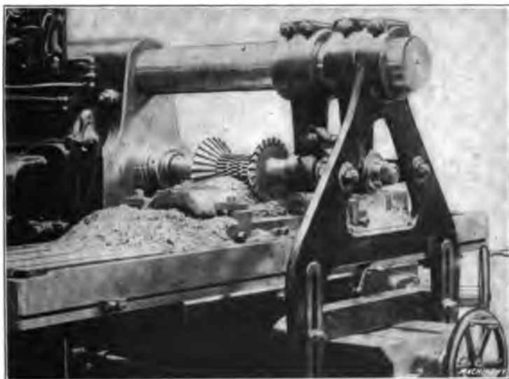
Fig. 23. Another Gang Milling Operation
