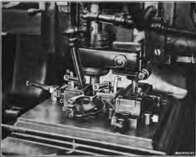
Fig. 16. Profiling Inside of Finger Lever for a Repeating Rifle
