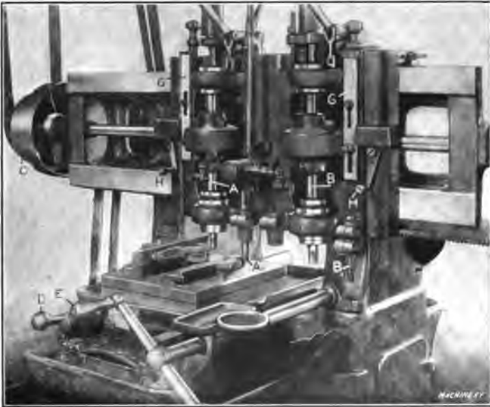
Fig. 15. Pratt & Whitney Profiling Machine Milling Rifle Trigger Guard
