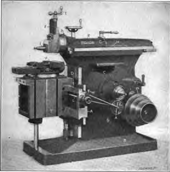
Fig. 1. Cincinnati Back-geared Crank-shaper
