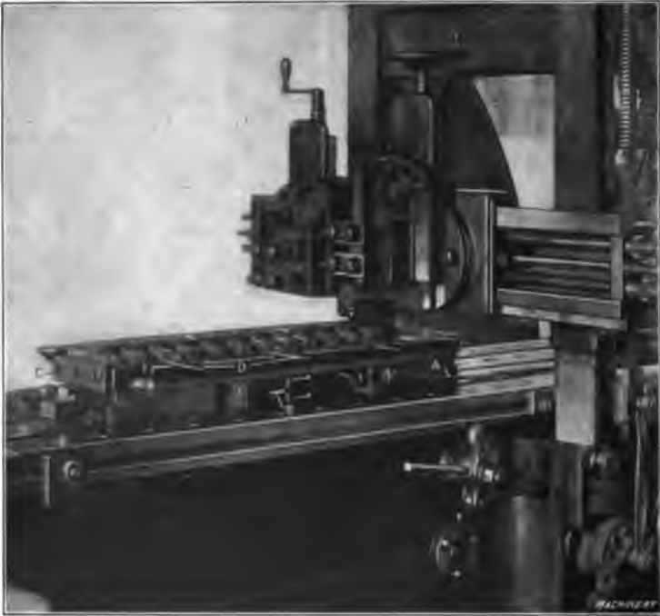
Fig. 25. Walker Magnetic Chuck applied to Planing Operation
