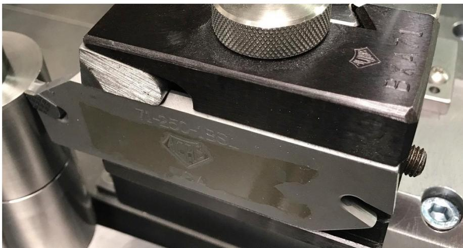
I often get asked about using HSS or braised-on carbide-tipped parting blades can be held in a holder like the Aloris 71. Look closely below at how this tool holder secures the parting blade in position. Notice that the blade clamping top and bottom is wedge-shaped to force the blade against the side of
