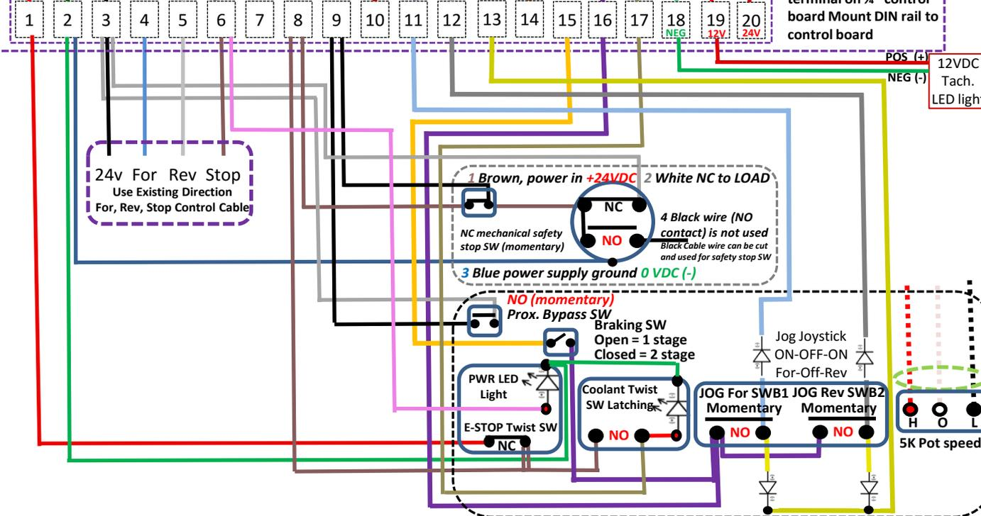
Belden Shielded VFD cable 8 conductor (18-24 AWG). Note: cable shield (drain wire) ground at VFD end only
