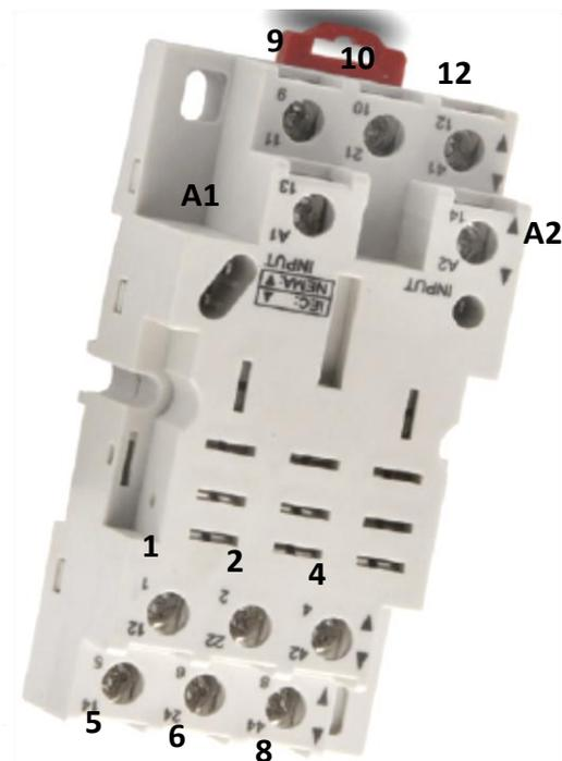
Note that relay connections on socket bases are different than the relay spades, connect via the labeled numbers on the relay socket base screw terminals. Note proper polarity and orientation of diodes and LEDs, the banded side is the (-) cathode which is the T in the diode diagrams.
