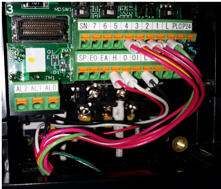
Use Star Grounding, Ground shields only at VFD end of cable.
