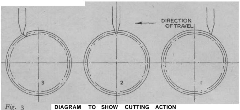
provide the feed, which in this case would have to be put on by hand after every cutting stroke.
