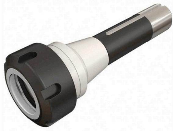
This is the ER40 collet chuck with MT3 arbor end that would fit the tailstock on a lathe, or in rotary table with MT3 taper.
