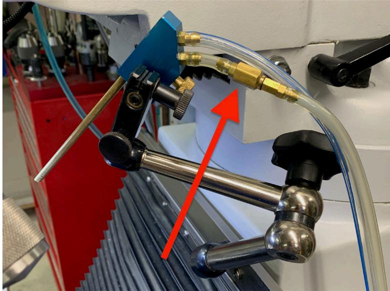
As you can also see from the photo above, I prefer to have my Fogbuster delivery nozzle and mixing control valve mounted on an articulated holder – in this case a spare Noga indicator holder that has been secured to a mounting bar I added to the mill column. Similarly, I prefer the same setup on the lathe, but using a magnetic base to provide additional positioning flexibility.
