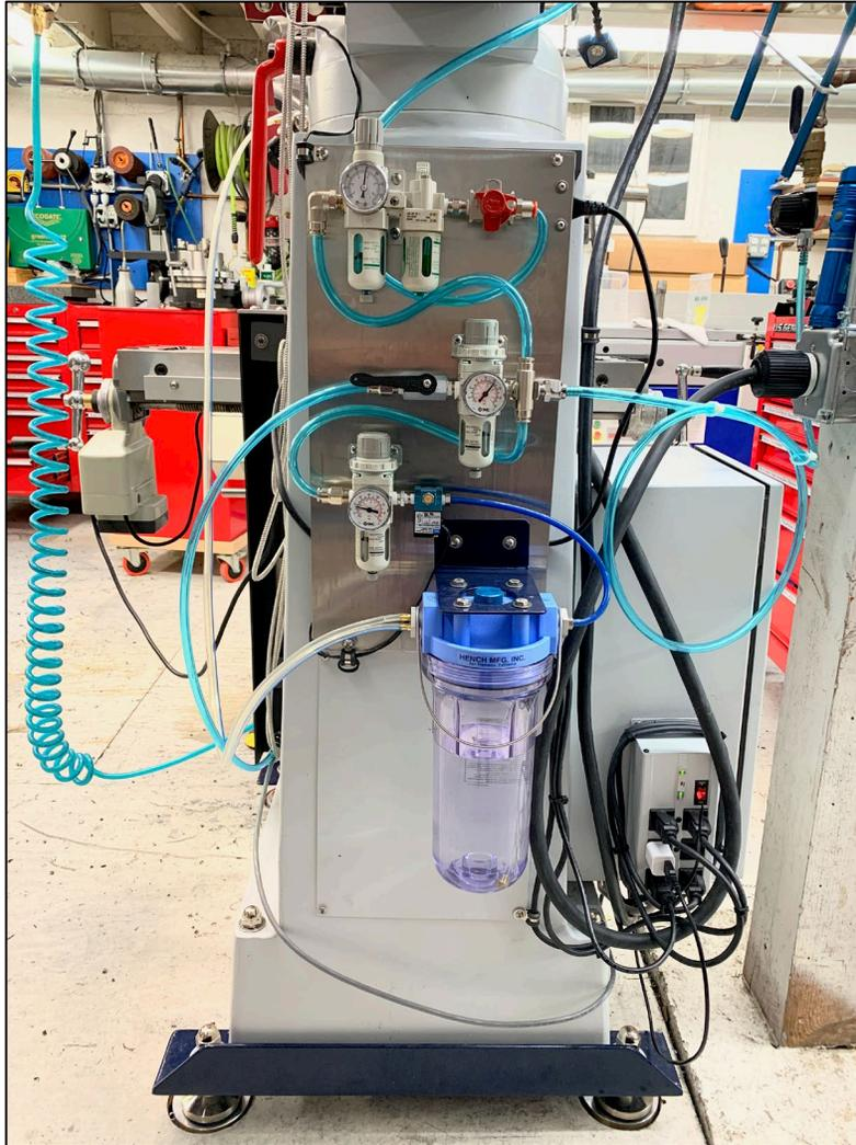
As you can see in the photo above, I have an elaborate compressed air control system as part of this installation. Air comes into the system from the right side of the photo to a 3-way splitter. The raw air at 160 PSI is delivered to three separate regulators.
