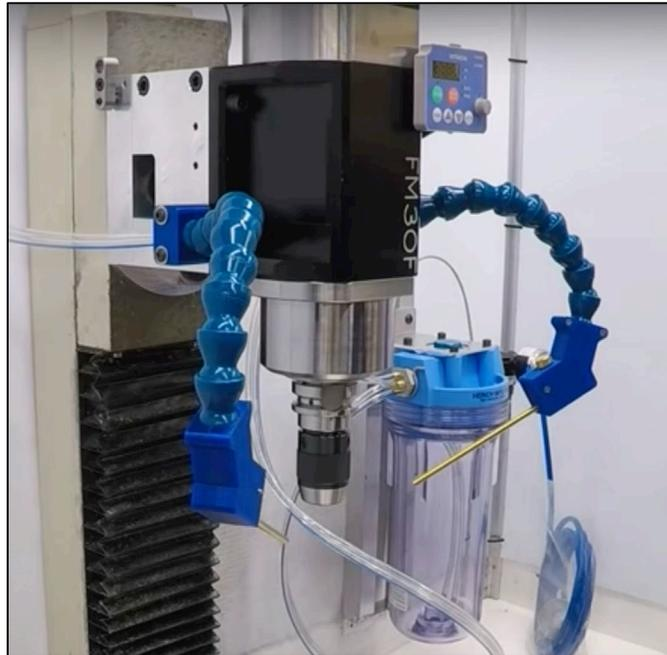
On both my mill and lathe, the Fogbuster is turned on/off with a switch integrated into the control system. You can see the coolant switches illustrated in the two photos below. If the coolant switch is on, the Fogbuster solenoid is triggered which delivers compressed air and coolant to the nozzle.
