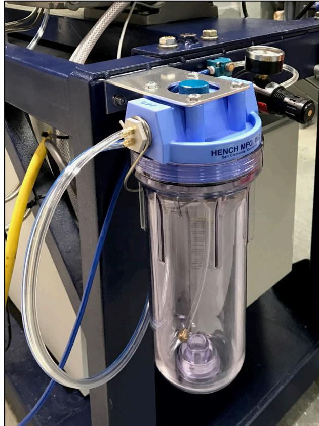
The Fogbuster kits come with the coolant canister, a regulator, an air switch, the necessary hoses, and the mixing and spray nozzle device with a simple magnetic-base stand as shown below.
