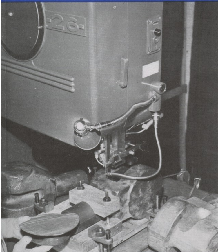
Above. Cutting long narrow slot. Note special set-up for holding work. Below. Precision sawing of openings in ends of long connecting rods.
