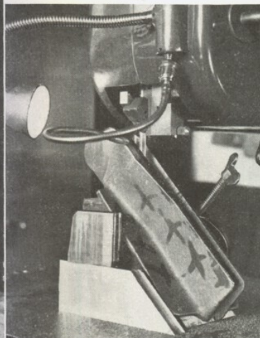
Above. Cutting long narrow slot. Note special set-up for holding work. Below. Precision sawing of openings in ends of long connecting rods.
