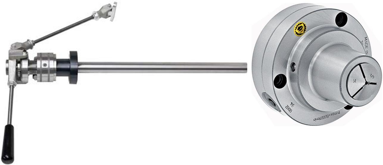
There are also square and hexagonal 5C collet blocks for holding round materials in a vise and indexing them at 60° or 90° similar to the ER40 collet blocks shown above. Here is a photo of square and hex 5C collet blocks. The black cylindrical item on the right is a quick-release collet closer and the handle actuates the collet from clamped to unclamped position.
