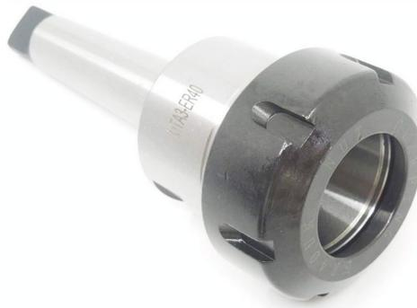
ER40 collet blocks are available for work holding small diameter round parts on the mill - the part is secured in the ER collet and then the blocks are then secured in a mill vise or the jaws of a conventional lathe chuck. This is one way you can hold cylindrical materials in a mill vise, and then rotate the collet block in the vise to perform successive operations that are clocked at 60°, 90°, 120°, or 180°. Shown below is a photo of a square and a hexagon ER40 collet block.
