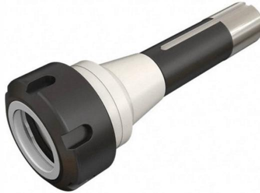
This is the ER40 collet chuck with MT3 arbor end that would fit the tailstock on a typical 12-14" lathe, or in rotary table with MT3 taper.
