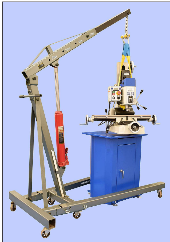
Figure 1-3 Lowering the mill into position
