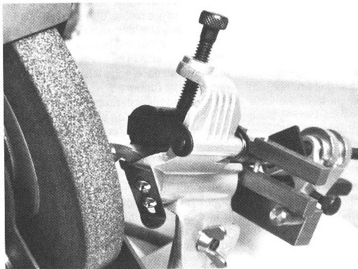
10 The parts in photograph 9 in use on the sharpening jig.
